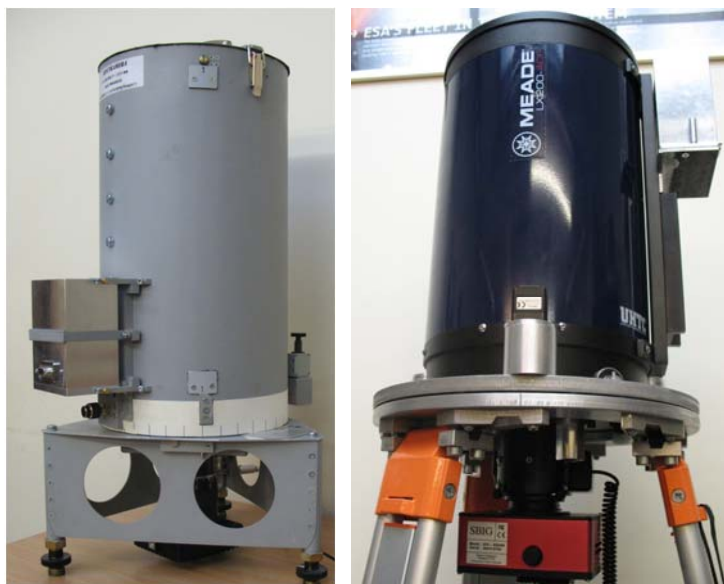
Figure 8. A prototype of a digital zenith camera (left) and final construction (right)
