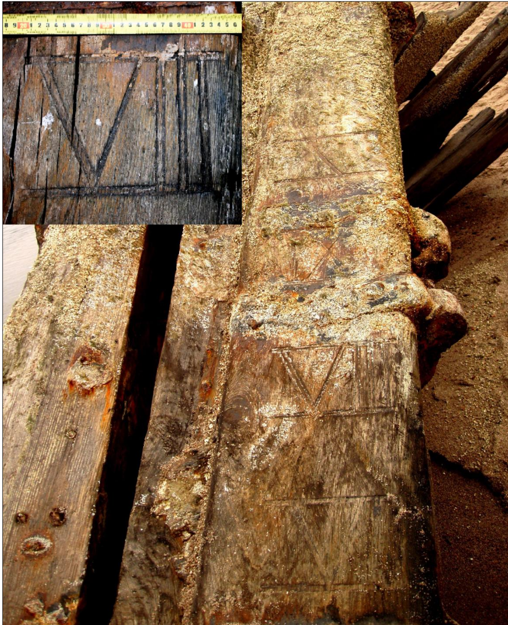
Figure 5. The scale of feet carved on the sternpost of the Melnragė wreck fragment. Photo by K. Perminas.
