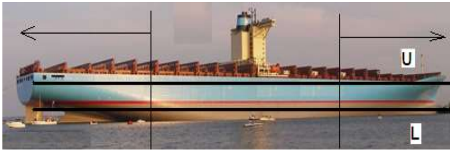
Figure 6. Illustration of water plane variation at ship's fore and aft part
